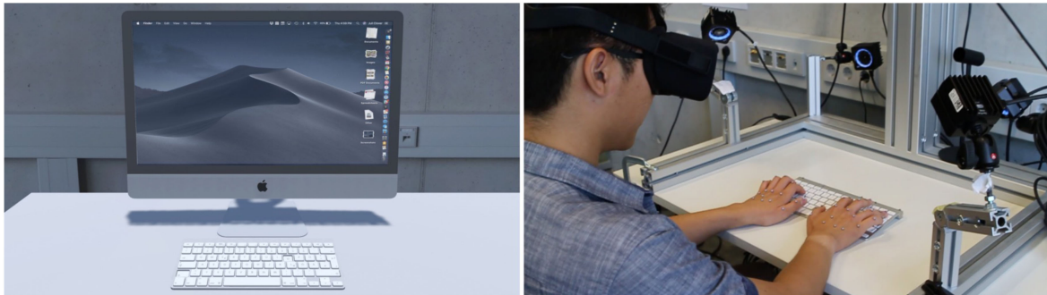
FIGURE 1. Left: A virtual office workspace resembling a physical one. Right: Stationary apparatus comprising a workstation, MR headset, and an accurate optical hand tracking system to enable text input in MR.
