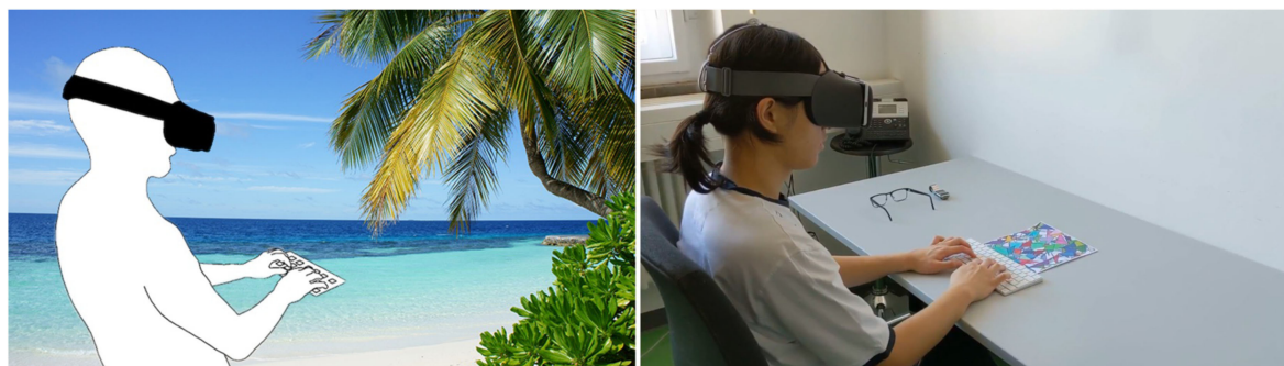
FIGURE 2. Left: Virtual office that is operated by a user outside of a physical office environment. Right: Lightweight, mobile setup comprising a smartphone, MR viewer, and physical keyboard to enable text input in MR.
